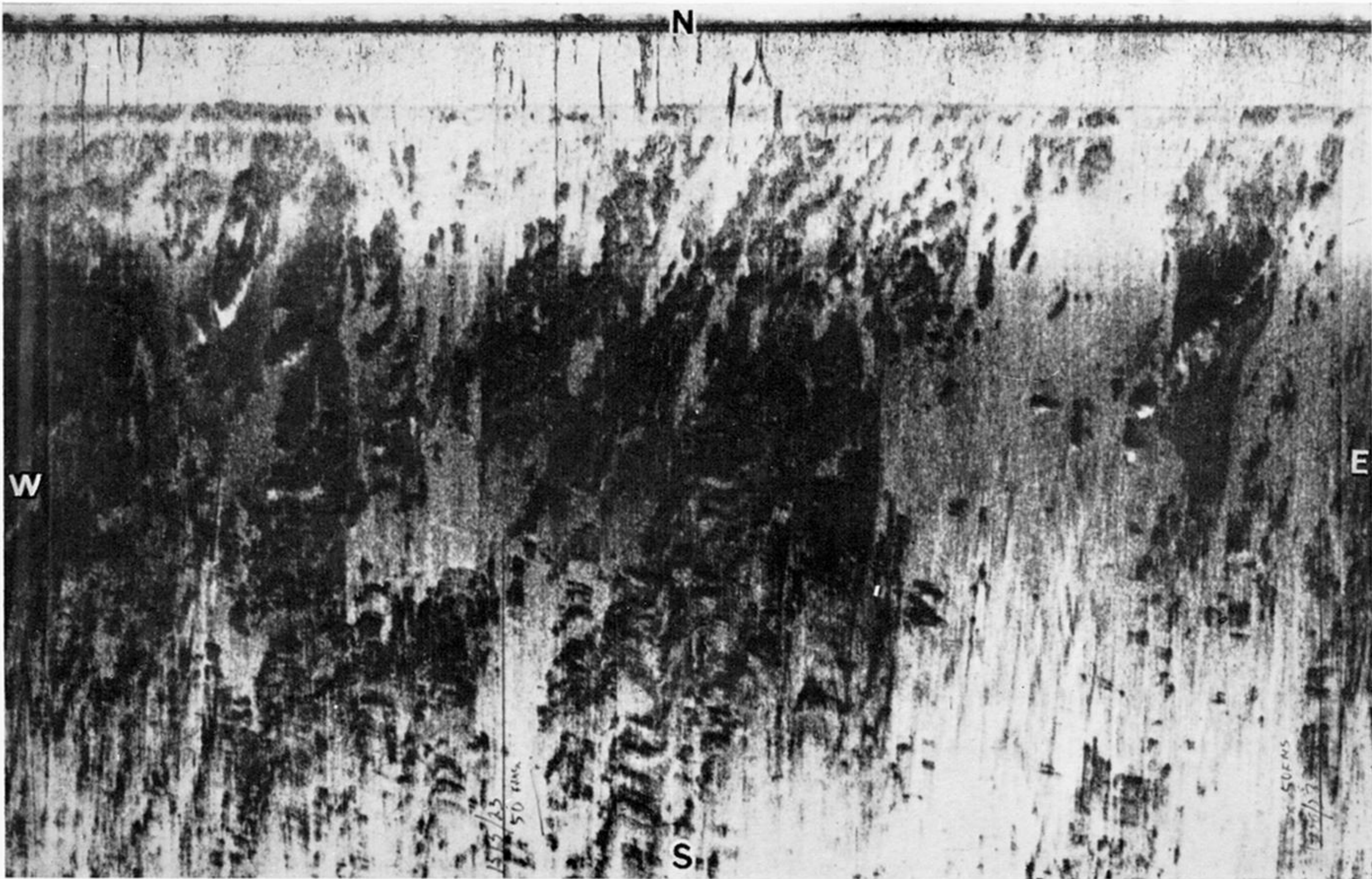
FIGURE 18. An acoustic map of 8 \times 1 km of sea floor west of Brittany (black rectangle in figure 17) showing ragged outcrops (dark tones), of Palaeozoic or metamorphic aspect, separated by flat, sandy floor.
